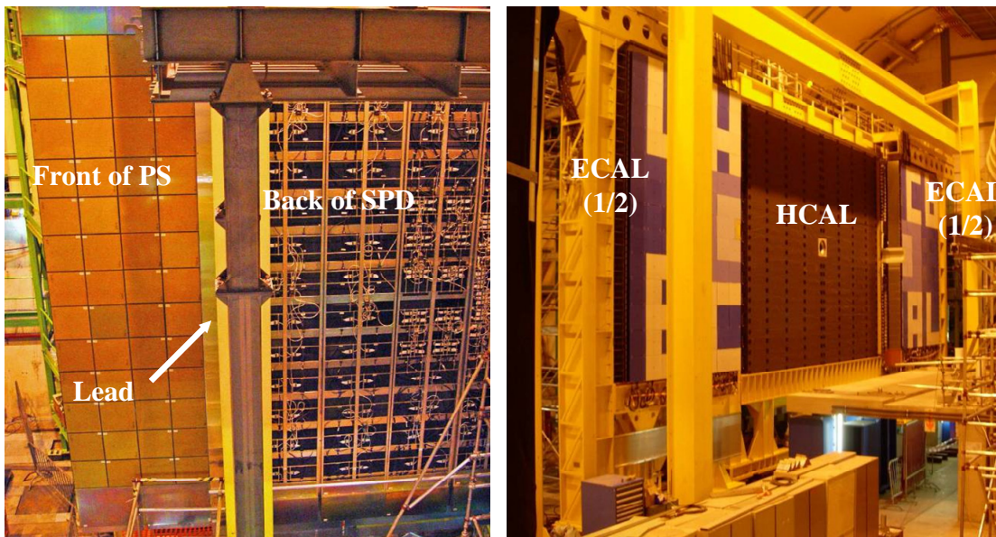
Figure 3-2. View of the calorimeter system. Left: PS and SPD. Right: ECAL (open) and HCAL before PS/SPD installation.
