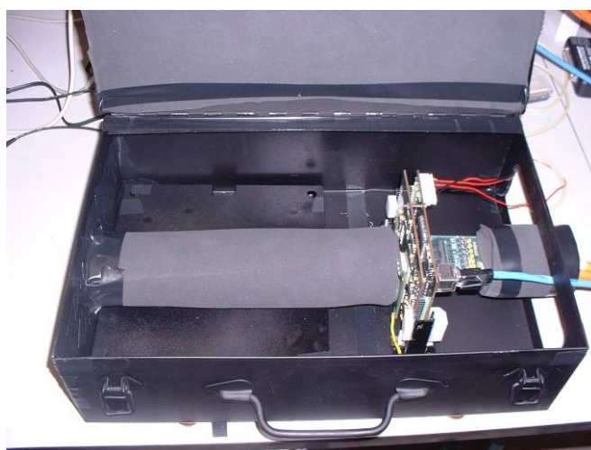
Figure 6-58. LED test set up for the VFE card.
