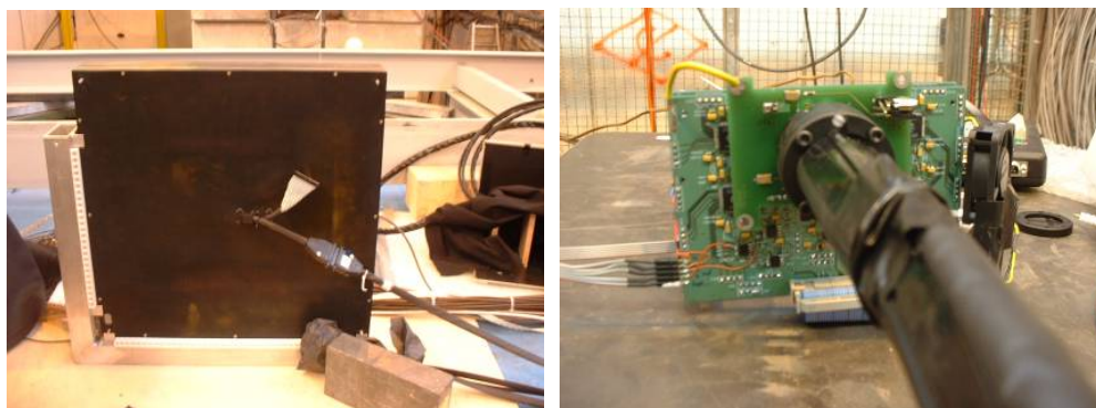
Figure 6-68. Photograph of the 4x4 SPD module (left) and of the VFE prototype (right).
