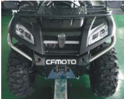
TYPICAL FRONT UP POINT LOCATION
