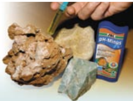
Check rocks for any possible lime content using a drop of JBL pH-Minus. If foam appears when a drop of JBL pH-Minus is added to the rock, the rock contains lime! Calciferous rock should not be used as it may increase the hardness of the water.
