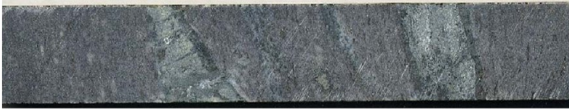
Skarn-banded intermediate metavolcanic rock. Vihanti mine, drill hole R1017, 55.60 m. Width of drill core 2.2 cm. From Luukas et al. (2004).
