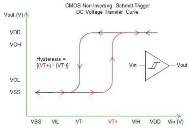
Figure 3: CMOS Non-Inverting Schmitt Trigger DC Voltage Transfer Curve
