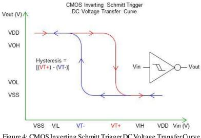
Figure 4: CMOS Inverting Schmitt Trigger DC Voltage Transfer Curve
