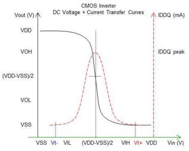
Figure 2: CMOS Inverter: DC Voltage + Current Transfer Curves
