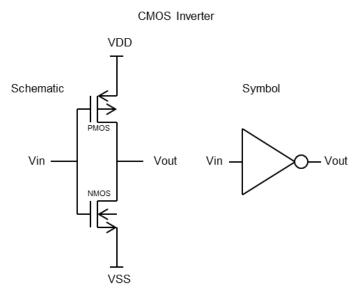
Figure 1: CMOS Inverter: Schematic and Symbol
