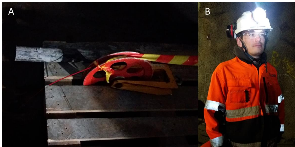
Figure 1. A) Fibre optic cable installed to act as a seismic sensor in a borehole in the Kylylahti mine. B) New postdoctoral researcher of the COGITO-MIN project at the University of Helsinki, Marko Riedel, participating in the VSP data acquisition work. Marko's postdoctoral research work will focus on the development of processing and interpretation methods for the acquired VSP data sets, in collaboration with Vibrometric.
