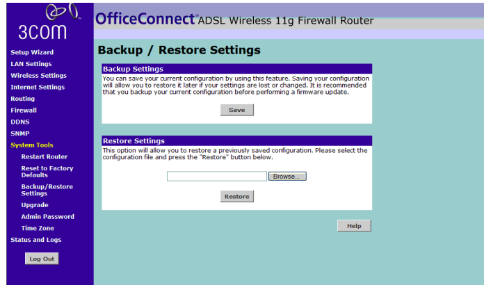
Figure 64 Backup/Restore Settings Screen
